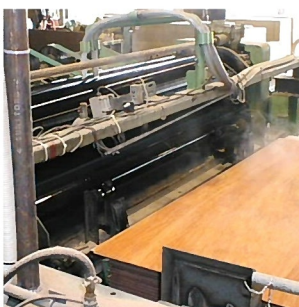
Coating by spray (generally used this method)
